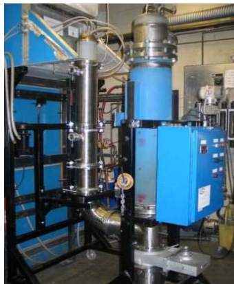
Figure 2.9. RF Plasma process, University of Sherbrooke (Simard 2006).
