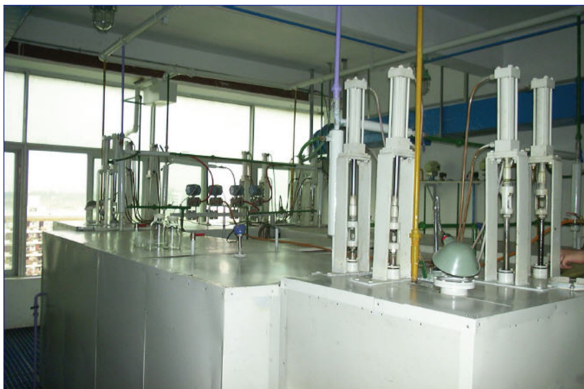
Figure B.11. Cycled CVD furnaces.
