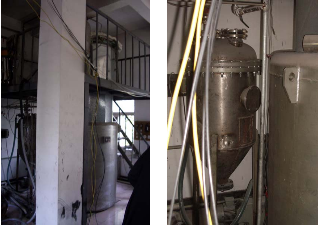
Figure 2.5. CVD-based fluid bed unit in stainless steel materials at Tsinghua University.
