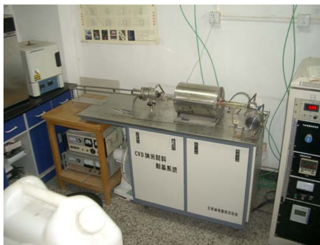
Figure B.8. CVD furnace (fabricated in-house — quartz tube) used to perform experiments related to growth characteristics and fluctuations of reaction temperature.
