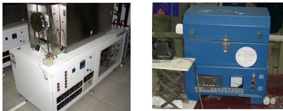
Figure 2.4. CVD-based quartz tube CNT units at research laboratories at Tsinghua-Foxconn Nanotechnology Research Center, China.
