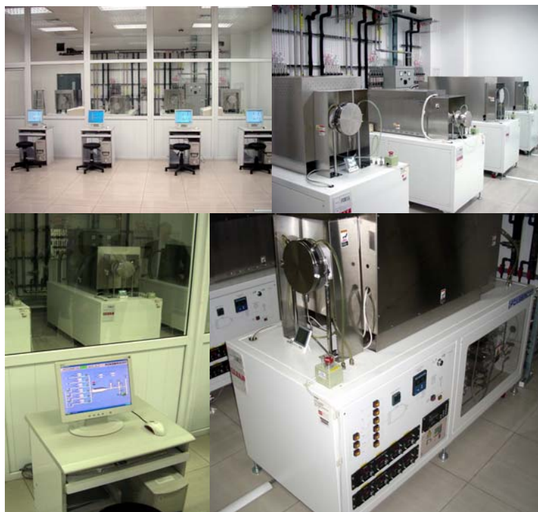
Figure B.22. Computer-controlled tube furnaces for CVD growth of CNTs and nanowires on full 4" wafer substrates. The furnaces are enclosed in a dedicated room, and the gases are stored in a separate room beneath the laboratory.
