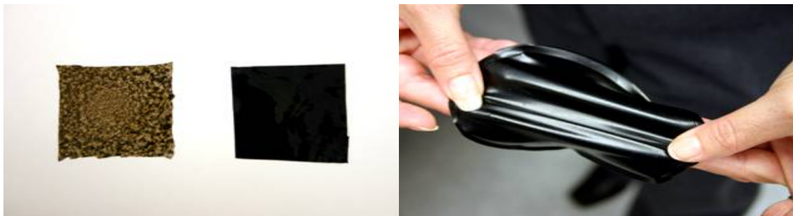
Figure 3.3. Example of poor (left) vs. good (right) dispersion of carbon nanomaterials in polyurethane films, and demonstration of stretching of well-dispersed CNT-polyurethane film (Banash 2006, 142).
