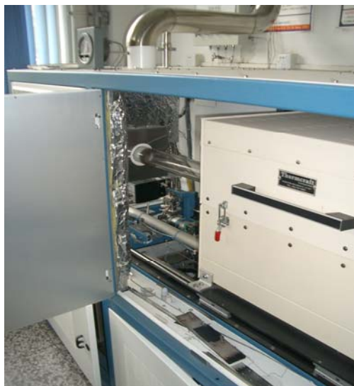
Figure B.9. Commercially procured CVD tube furnace with integrated atmosphere control.
